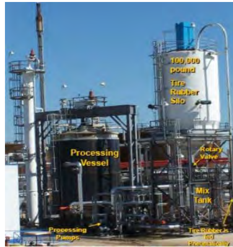
Terminal Blending Process for Rubberized Asphalt
